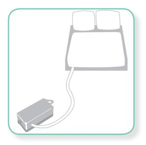
• Connect the pump plug to the digital timer. Insert one end of the hose into the hose connection to the side of the pump and connect the other end to the pressure regulator on the upper part of the vacuum extender.
